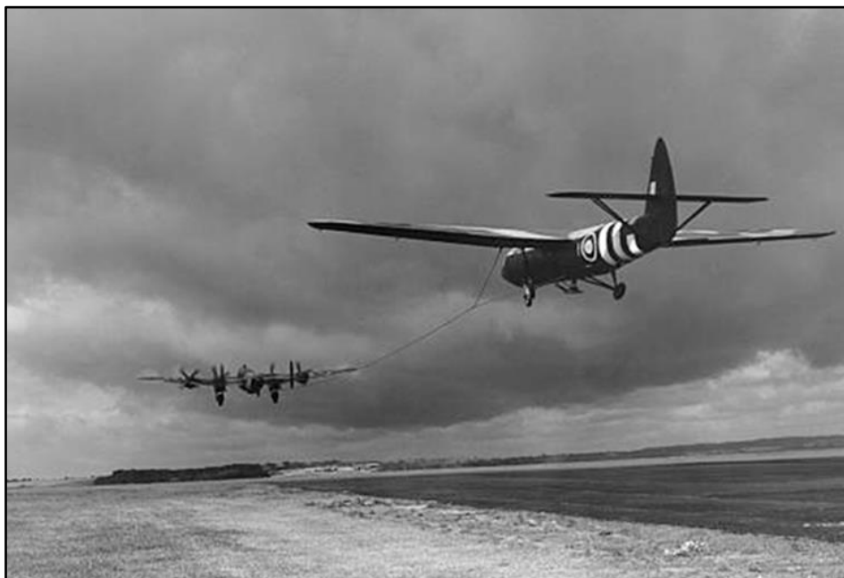
A Halifax V with an Aircspeed Horsa taking off from RAF Tarrant Rushton.
